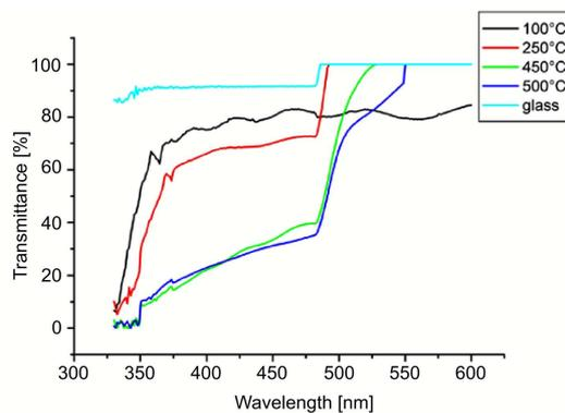
Fig. 3. Transmission spectra from UV-VIS measurements
