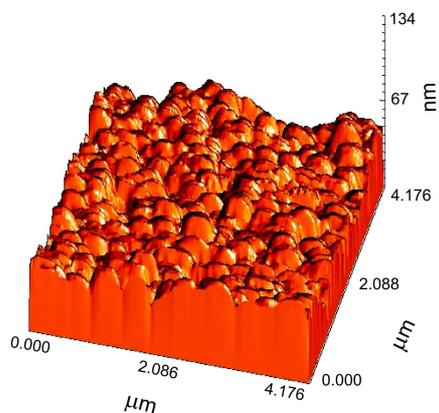
Fig. 2. AFM picture of the film deposited at 500°C.
