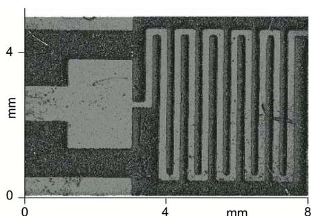
Fig. 1. Picture of special platinum electrode.
