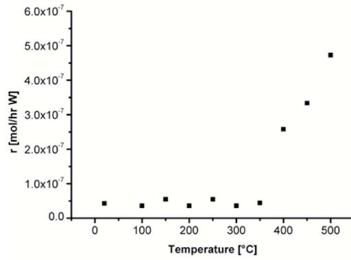
Fig. 4. Variation of photocatalytic degradation speed with deposition temperature
