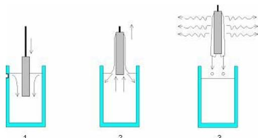
Figure 1. Scheme of method dip-coating, 1 – dip the substrate into the sol of precursors, 2 – take out the substrate from sol, 3 – evaporation of solvent from substrate surface
