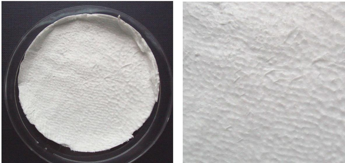
**Figure 4:** Nanofiber web from J18 polymeric solution
